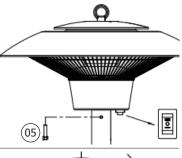
Step 5: Fix the power cable into the groove in the base bottom using the pressure strips and screws.
